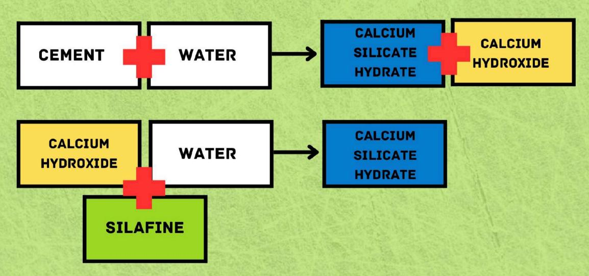
Silafine, a pozzolanic material, reacts with calcium hydroxide and water to form more calcium silicate hydrate (CSH), which binds aggregates and reduces calcium hydroxide content. This reaction strengthens the concrete matrix, lowers permeability, and enhances durability by minimizing calcium hydroxide.
